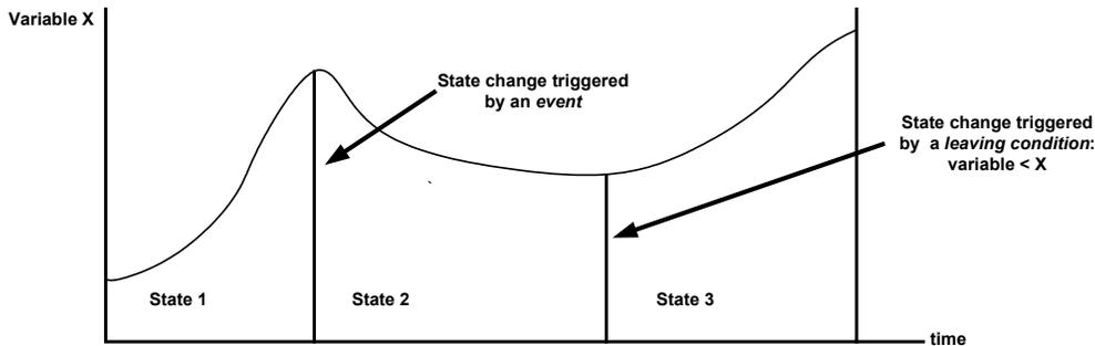
Figure 2: continuous variable in a hybrid machine
